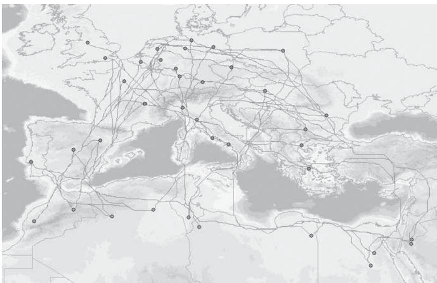
**Figure 1:** Potential Configuration of HVDC lines connecting EU demand centers with CSP sites in MENA.
